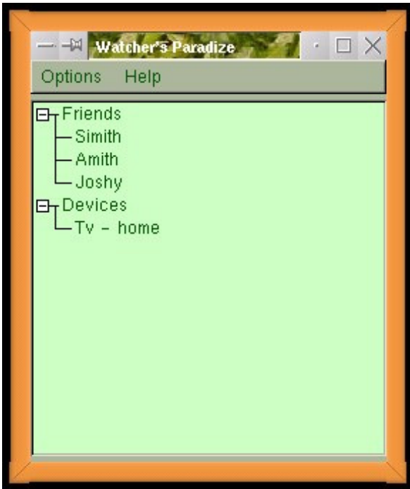
Fig. 2 (above): A snapshot of the SIP User Agent, when the TV comes online.
